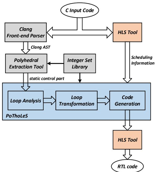
Fig. 6: Tool flow for code transformation framework.
