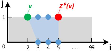
Fig. 5: The calculation of  $d(v)$  for the example loop shown in Listing 4. Each dot is one integer point and represents one iteration. If we count after iteration  $v$ , there are 6 points including  $Z^p(v)$  in the blue area when  $v = [2, 1]^T$  and  $m = 1$ .
