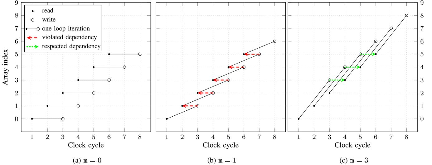
Fig. 1: The impact of the undetermined variable  $m$  on fully pipelining the loop shown in Listing 1. We assume that  $N = 6$ , and the iteration latency is 3 cycles.
