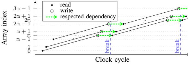
Fig. 2: Breaking the pipeline execution at  $(m+1)^{\text{th}}$  and  $(2m+1)^{\text{th}}$  iterations, when the loop shown in Listing 1 is running at initiation interval of one cycle.
