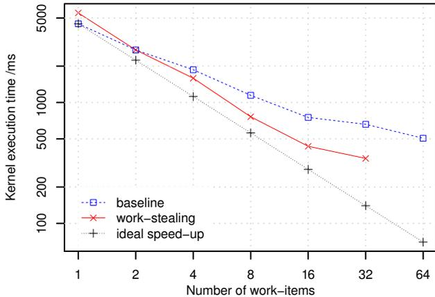
Figure 4: Kernel execution time for the filtering algorithm.
